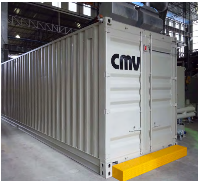
Blast room in container.
