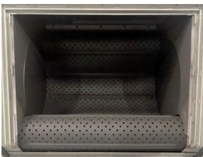
ET-80 internal view of the blasting chamber.
